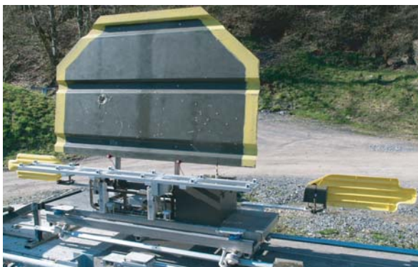
Example: tank target mounted on moving carrier (1 tank target "CB2" + LOMAH, 2 infantry targets "CF3U" on the side)
